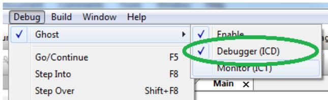
To enable in circuit debug (ICD) mode, select the Debugger (ICD) dialog from the Flowcode Debug->Ghost menu.
