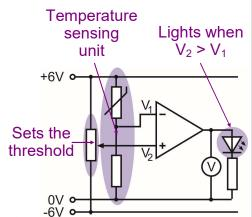
Near the switching threshold, any electrical noise could push the signal over the threshold, and cause the output to switch rapidly on and off, from the noise alone. Then, it may be better to use a Schmitt trigger circuit.
