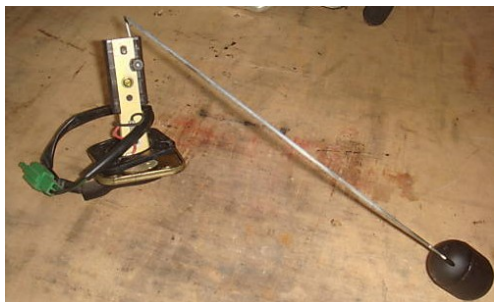
Fuel sensor with float
