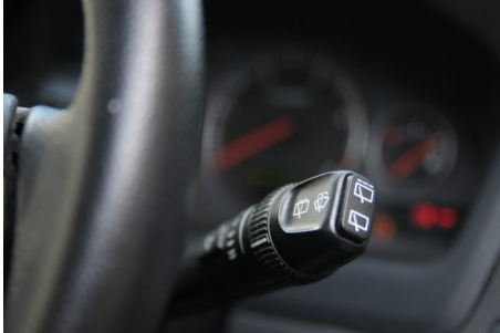
Indicator stalk houses several types of switch
