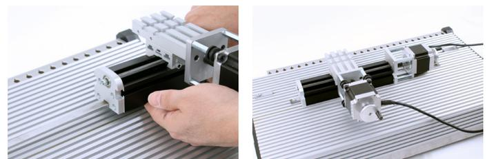
Tighten both screws to hold the Cross Slide module securely in place.
