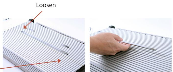
Slide the Cross Slide module onto the long retaining bar. Position the Cross Slide module centrally on the platform.
