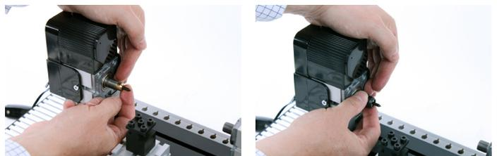
Loosen the screws in the tool holder and place in the cutting bit, use the small brass shims (1mm, 0.4mm, and 0.1mm) to adjust the height of the bit. The bit needs to be in line with the centring bit. Secure the cutting tool into the tool holder by tightening the tool post screws.
