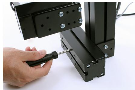
Next tighten the four screws located on either side of the Tool Post.
