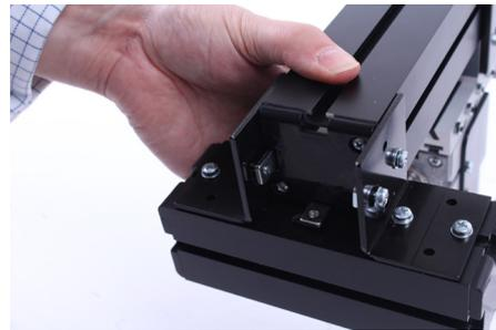
Carefully place the assembly onto a flat surface. First tighten the two screws located on the inner face of the Short Machine Bed, you will need to insert the screwdriver into the short machine bed as shown opposite.
