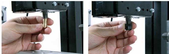
Place the collet into the motor assembly and secure in place using the collet holder; do not tighten
