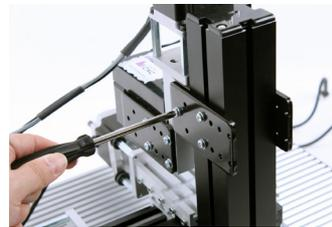
Hold the Cutting Tool Head securely while loosening the Connection Piece located between the Tool Post and the Small Cross Slide/Motor Assembly.
