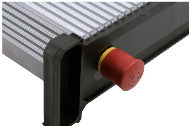
Matrix MicroCNC machines provide two methods of initiating and emergency stop. These are a 'Physical' emergency stop button located on the right hand end of the Controller Base Plate and a 'Software' emergency stop within the control software. The software emergency stop will be covered later in this document.
