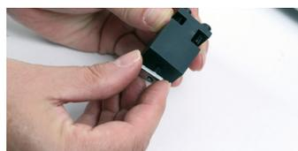
Assemble the Tool post using the M4x70 socket head screw and a slot nut from the accessory pack.
