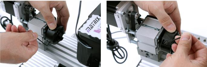
To secure a workpiece into the 4 Jaw Chuck use the 2mm Allen key to adjust the position of each Jaw individually, there are guide lines on the face of the chuck to help centralise the workpiece.
