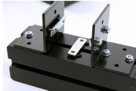
Slide the Tool Post & Motor Assembly onto the Short machine bed ensuring the three clamping plates locate into the T-slots of the Tool Post. The Short Machine Bed should be positioned underneath the Motor.
