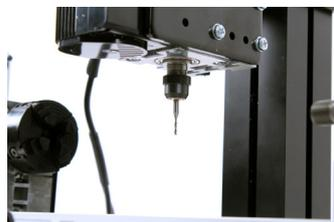
Insert the cutting bit into the collet and tighten the collet holder until the cutting bit is held in place
