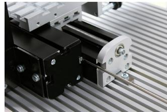
Insert the small retaining bars into either side of the Lathe module and tighten screws
