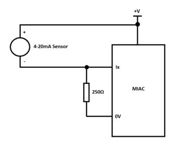
This circuit demonstrates how a 2-wire current loop device can be connected to an ADC input, such as that of the MIAC.
